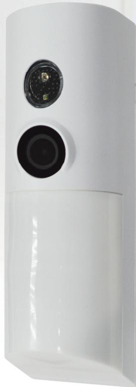
The SV201 PIRCAM is a detector combining Passive Infra-Red (PIR) sensor and image sensor to capture images when motion is detected. This is used for video verification at an alarm monitoring center to reduce false alarms events triggered from the protected site. The device also supports on-demand photo capture by the controller, as requested by a user through the App, or as an action following an alarm condition or perhaps as part of a home automation scenes.
